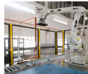
AUTOMATED CONVEYING, BOXING, WEIGHING, SORTING, STORAGE AND PALLETISING SYSTEM
